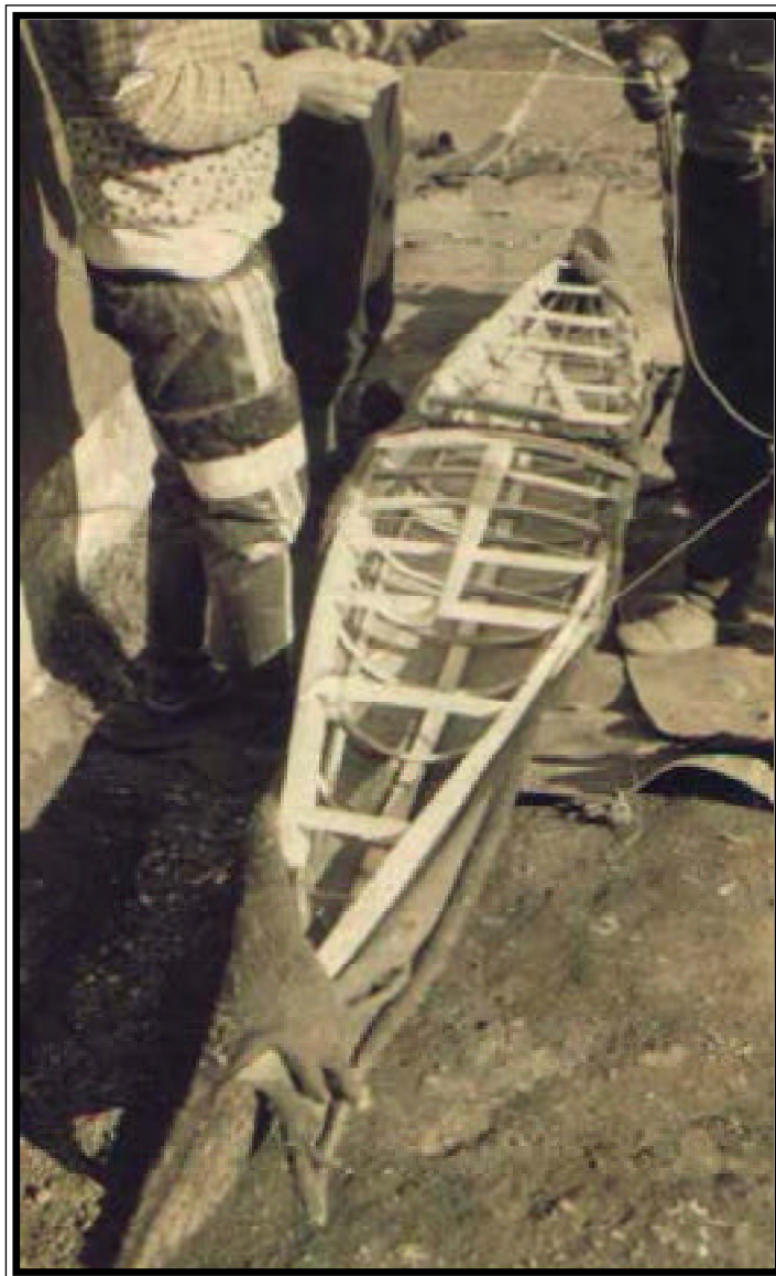
Greenland, Igdlorssuit, 1959. Kenneth Taylor's made to measure kayak in the process of being covered with seal skins. Photo: courtesy of Alan Byde.
