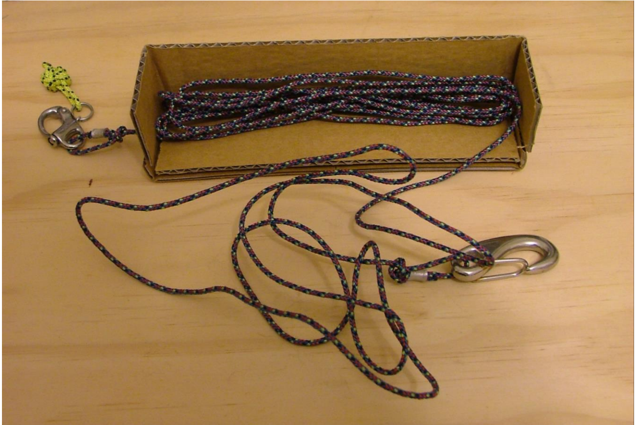
2 Zigzag the line without coiling or figure eighting into a box as a length guide
